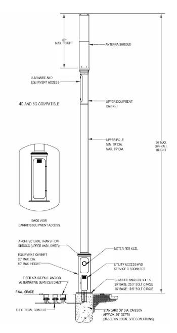
Figure 5-3: Freestanding Small Cell Assembly
