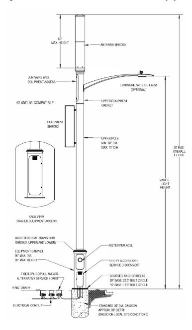
Figure 5-2: Combination Pole with Antenna and Equipment Shroud
